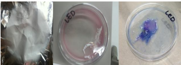
Fig. 5. Comparison between the state of the PVDF membrane before the experiments (left), after 5 days of cell growth (center) and after 12 days of cell growth and a blue methylene staining (right).
